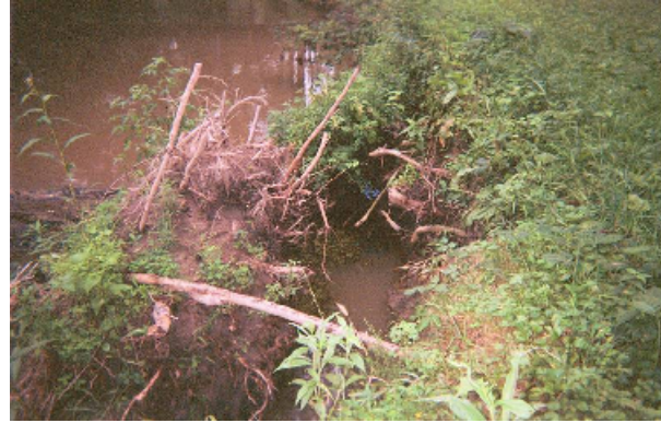
Photograph 2: Erosion from Diverted Flow at Root Mass
