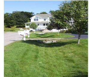
**Grassed Filter Strips:** Low-angle vegetated slopes, usually located adjacent to parking areas and other large impervious surfaces, that slow flows and treat stormwater.
