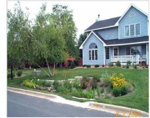
**Vegetated Swales:** Shallow drainage channels usually located adjacent to roadways (as an alternative to typical curb and gutter treatments) used to convey and filter stormwater.
