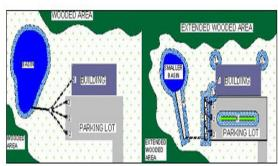
Illustration from DEP Stormwater BMP Manual showing LID alternative to typical commercial development
