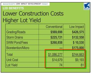
Example of Construction Cost Analysis of Conventional versus LID Development
