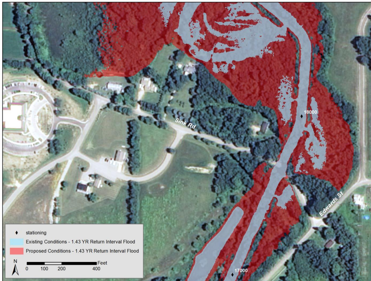
Figure 64. Plan view of the water surface extents around Sink Rd. at the 100-year flood. The proposed (red polygon) water surface rises and covers a larger area than the existing (blue hatched polygon) area.
