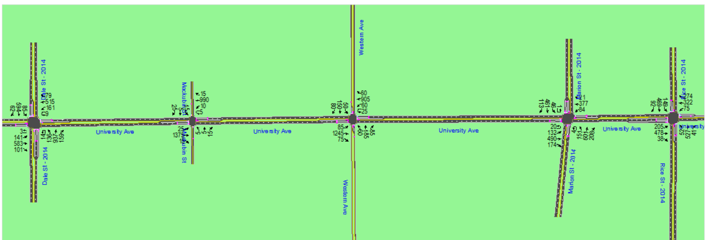
TDG performed Synchro analysis for 15 intersections along the University Avenue Corridor
