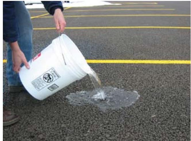
*Water on Porous Asphalt*
