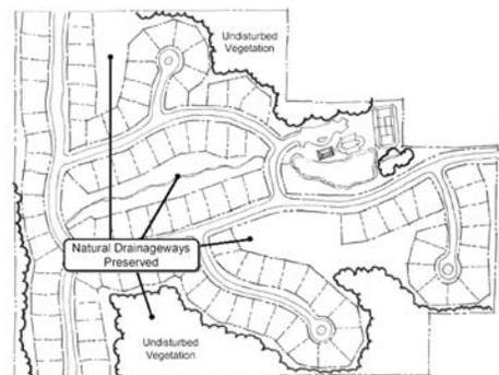
*Schematic of a site design protecting natural drainage features*
