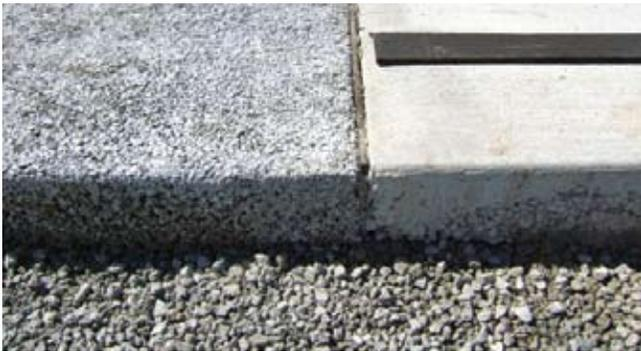
*Pervious and impervious concrete*
