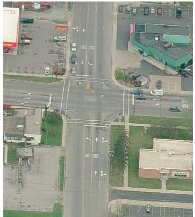
Aerial view of the intersection of Napier Ave. (left-right) and Colfax Ave. (up-down), showing a crossing width of five lanes on each side of the intersection, with a school building shown to the lower right
