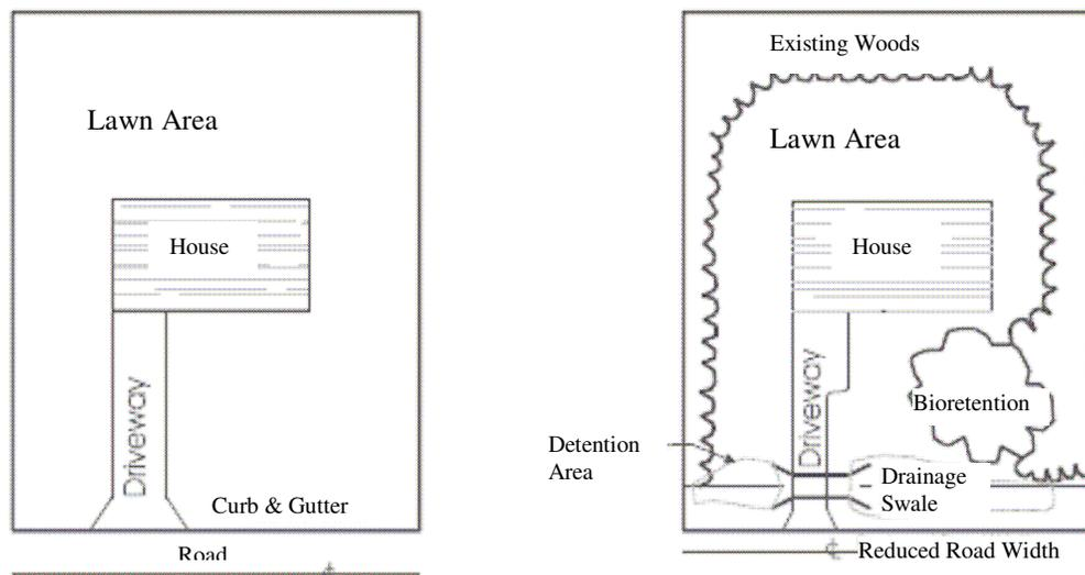
**With Conventional Development** water is moved off site as quickly as possible with curb, gutter, and storm sewers.
